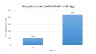
Inspecting a turbine blade takes ca 20 seconds with NAW® inspection. The result is a "damage value", a calculation of the total amount of damage in the part that determines whether the blade can be used again or not. If inspecting same turbine blade regularly a damage progression can be calculated estimating remaining service life for individual blades.
