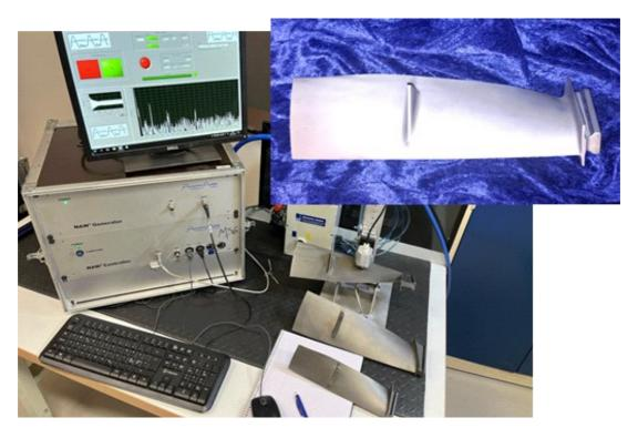
damage starts as rifts in the materials grain structure "audible". structure, when rifts grow together a crack has developed. Cracks and rifts in a structure carries sound different to a undamaged structure, the damages create anomalies in sound that can be measured.
