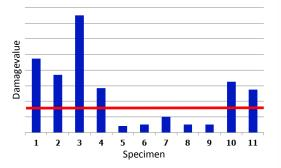
result. The specimens 1-4 and 10-11 contained damage of various severity. The specimens 5-9 were considered intact and had only negligible defects.
