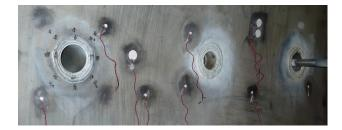
he NAW<sup>®</sup>-technique is a fast, reliable, easy-to-use non-destructive testing method. It is flexible in terms of geometry and material and is a strong challenger and complement to conventional methods. Since all evaluation is done by the software the NAW<sup>®</sup>-method is suitable for automated inspection in production lines as well as structural health monitoring.
